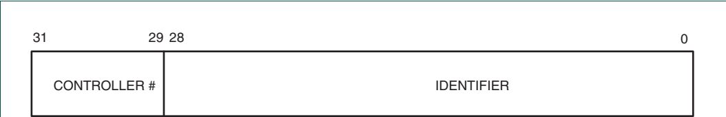
Fig 81. Entry in either extended identifier table
