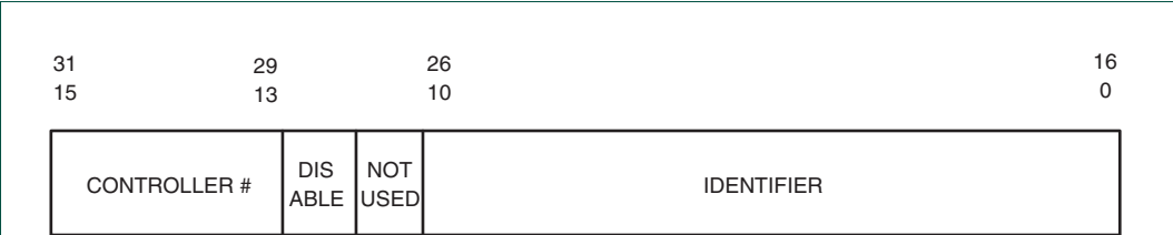
Fig 79. Entry in FullCAN and individual standard identifier tables
