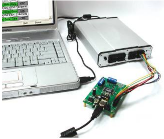
Fig. 2-6: An Assembly of Laptop, Logic Analyzer, and a Testing Board
