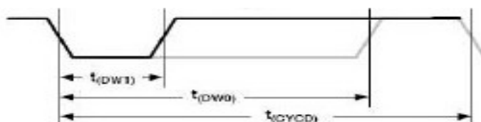
Fig4-113 - Signal from BQ-HDQ to Host
