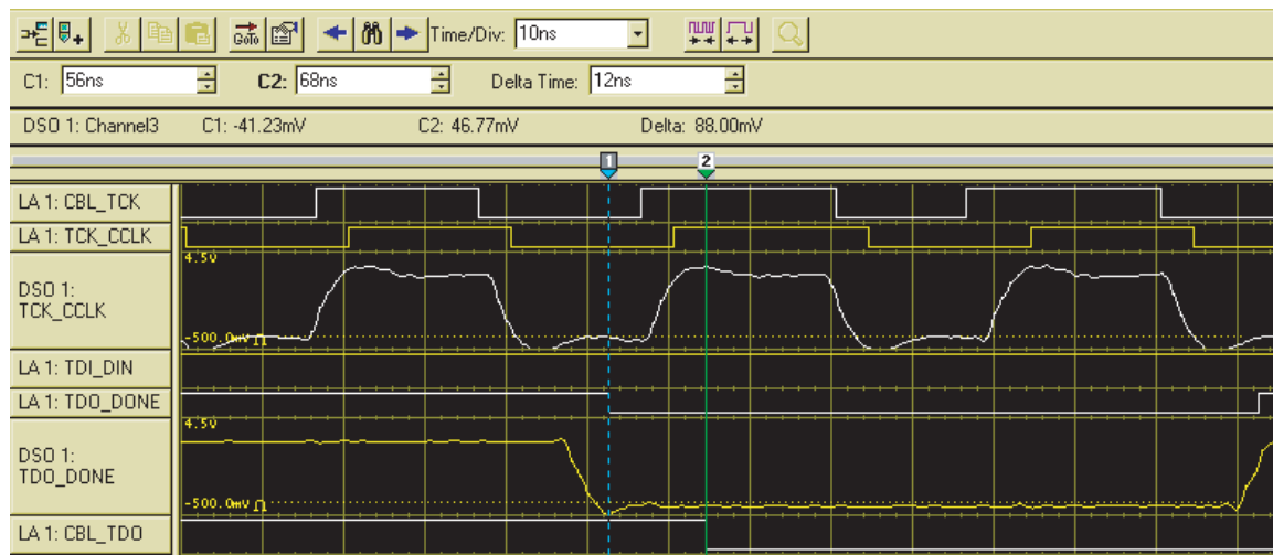
Figure 21: TDO_DONE_MISO Timing with Respect to TCK_CCLK_SCK (TDO_DONE_MISO to CBL_TDO Delay)
