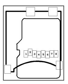
Notice that the pad numeration is written at the bottom of STM32-E407 under the microSD card connector.
