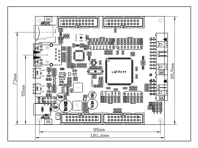
The three highest elements on the board in order from the tallest to the shortest are: capacitor C50 - 17.2mm (0.677") over the pcb; LAN connector - 13.6mm (0.535"); capacitators C42 and C48 - 11.5mm (0.453").
