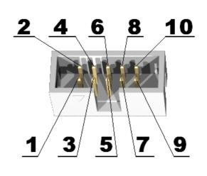
UEXT is a universal OLIMEX connector with 3.3V power supply and UART, I2C and SPI interface. Other device or modules with these interfaces can connected with UEXT. For example: MOD-NRF24L, MOD-RFID125, MOD-MP3 and many other are on the way
